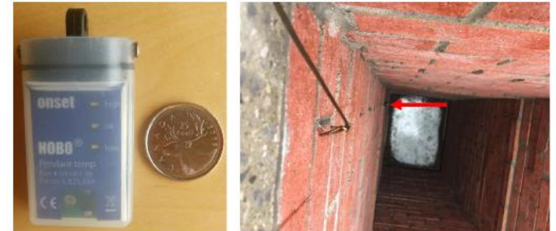
Figure 2. HOBO Pendant Temperature Data Logger deployed in structures occupied and unoccupied by nesting Chimney Swifts in 2017 and 2018 in Ontario, Canada (left). Example of data logger positioning inside a structure (right).
